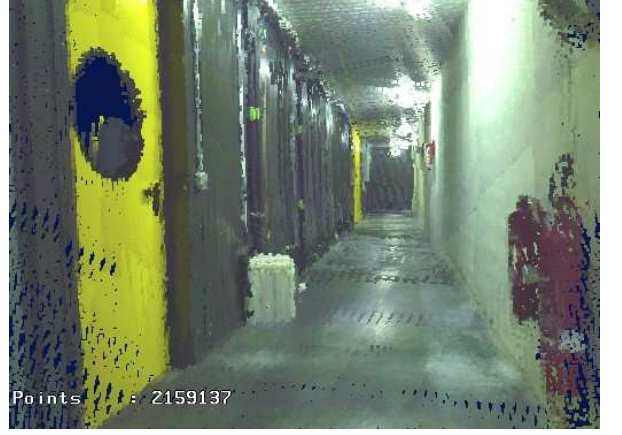
Fig. 3. Data recorded with the mobile robot Zora in a corridor environment at CS Department in Freiburg. The whole data set, which consists of 2,159,137 points has been registered using the ICP algorithm. Note the highly accurate color labeling of the individual 3d points, which is due to our calibration algorithm.
