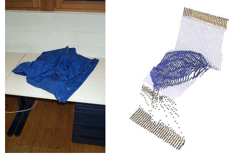
Fig. 6. A blue jacket lying on a desk. Photograph of the scene (left) and 3D scan acquired with Zora (right)
