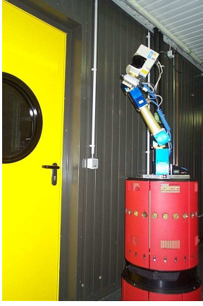
Fig. 2. The mobile robot Zora used for the experiments described in this paper. The robot carries a color CCD camera and SICK LMS range scanner mounted on top of a 4DOF AMTEC arm for flexible colored 3d scanning.
