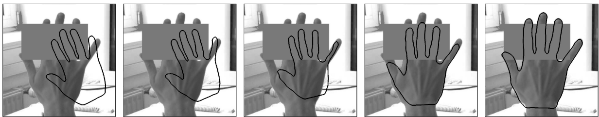
Figure 7: Gradient descent evolution of a parametric curve from initial to final with similarity invariant shape prior. The statistical shape prior permits a reconstruction of the hand silhouette in places where it is occluded.
