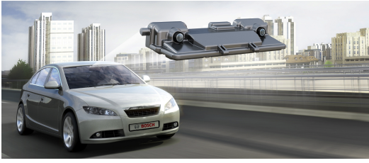
Fig. 10. The Bosch stereo video camera detects objects’ height and distance as well as capturing standard video images.
