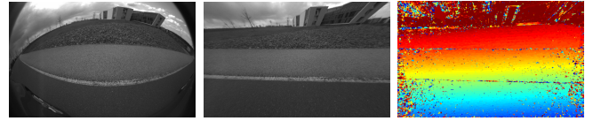
Fig. 6. Depth map computation—perspective images (middle) are rendered from the fisheye images (left) and plane sweep stereo matching is used between three temporally consecutive images to produce a depth map (right) for each camera at each time.
