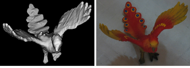
Fig. 5: Intensity-coded backprojection area element \mathcal{J}_i^\pi and corresponding input image. Some errors in the input geometry are clearly visible - no good texture can be expected in those regions.
