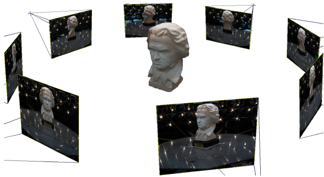
Fig. 2: Input images and geometry. Multiple cameras capture a static object. Each surface patch is visible in several input images, enabling texture super-resolution.
