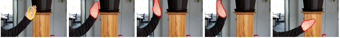
Figure 6. Moment constraints for object tracking. The user initializes the tracking by clicking an ellipse in the first frame, the moments of which constrain the segmentation in subsequent images. A small deviation of the centroid is allowed to track the moving object. Note that this approach is generic, as no shapes have to be previously learned.
