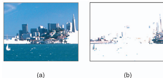
Fig. 15. Segmentation computed with the Fiedler vector thresholded at the median for the image from Fig. 14a: Separation into spatially coherent parts fails completely.
