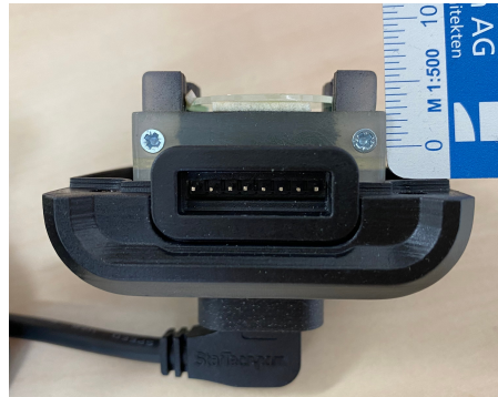
Fig. 3: The infrared filter is mounted parallel to the sensor, at a distance of approximately 2 millimeter. The sensor plane is located approximately at the 5 millimeter mark of the ruler.
