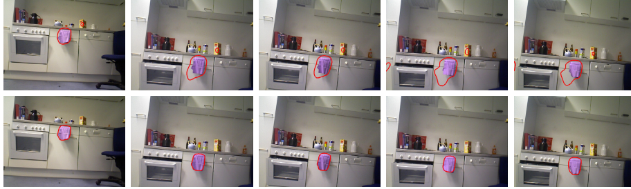
Fig. 2. Comparison of tracking an object with and without area constraint. Top row: Color-only tracking. Bottom row: RGB-D tracking: The surface area is constrained on the absolute dimension via additional information from the depth images.
