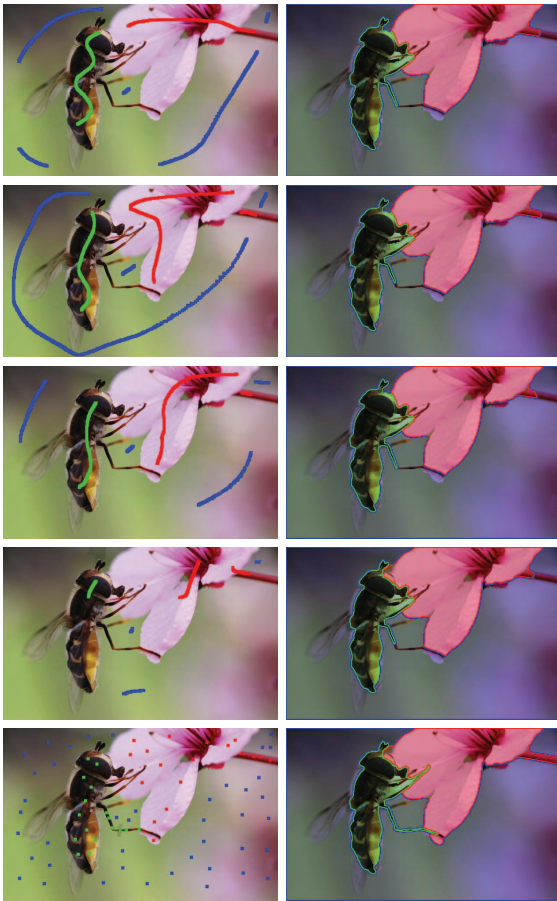
Fig. 16. Segmentation results for different scribble amounts and locations. The results show that the algorithm is not very sensitive to the user input provided the scribbles are placed in reasonable locations to well represent the color variation in the image.
