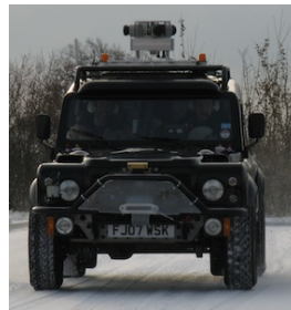
Fig. 2: Our robotic car, equipped with a 3D laser range finder on the top of the roof.
