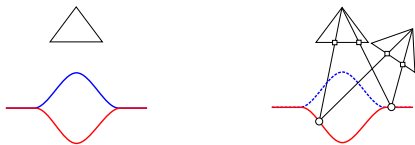
Figure 2: Shape-from-shading suffers from the concave/convex ambiguity (left). We introduce a practical approach to SFS under natural illumination, which achieves unambiguous 3D-reconstruction when sparse correspondences between multi-view images are available (right).
