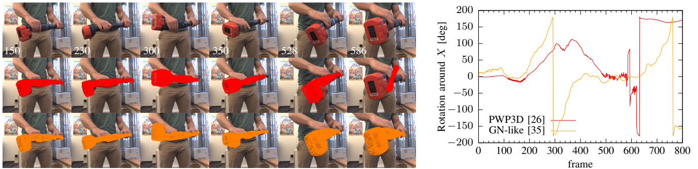
Fig. 8. Left: Visual results of a pose tracking experiment, where a hand-held screwdriver was rotated 360^\circ around its X -axis (top row: examples from the input sequence with the frame numbers depicted, middle row: results of the original first-order gradient descent implementation of PWP3D [26], bottom row: results of the Gauss-Newton-like optimization of [35]). Right: A corresponding plot of the estimated rotation around the X -axis for both methods. While the oscillations around frames 105–150 and 500–600 indicate that the gradient descent time steps are already near the limit of stability, the algorithm cannot reliably estimate the full 360^\circ rotation leading to a failure of PWP3D (see last frame central row).
