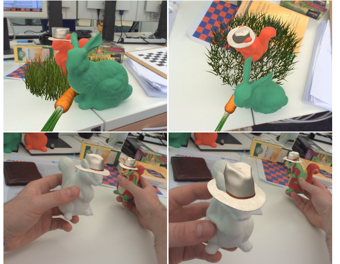
Fig. 11. Mixed reality visualizations in two different complex scenes with two tracked objects each. Based on the pose estimates, the real objects are augmented with virtual attachments (hats, a carrot and a patch of grass) in real-time. Here, despite large perspective changes and both modelled and unmodelled occlusions, the augmentations remain precisely in place. This makes our method very attractive for complex mixed reality systems.
