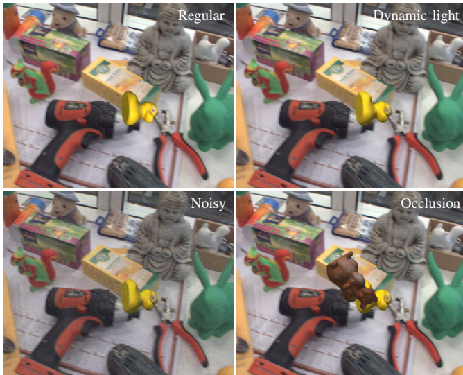
Fig. 10. An example frame from the RBOT dataset with the duck model in the four different variants. Visually comparing the regular with the dynamic light version clarifies the impact of the lighting aspect on the appearance of the object region.
