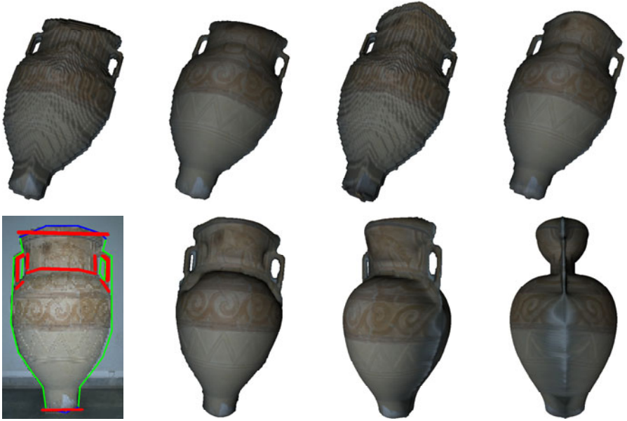
Fig. 3. Top row: height maps and corresponding reconstructions with and without marked sharp contour edges. Bottom row: input image with marked contour edges (blue) and line strokes (red) for local discontinuities which are shown right.
