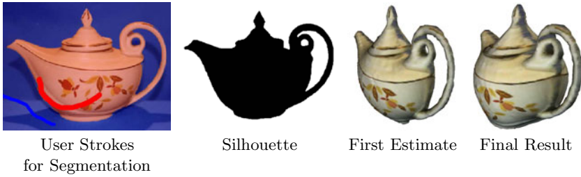
Fig. 1. The basic workflow of the single view reconstruction process: The user marks the input image with scribbles ( left ) from which a silhouette is generated by segmentation ( second from left ). A first reconstruction estimate is generated automatically from the silhouette ( third from left ). The user can then iteratively adapt the model in an interactive manner ( right ).
